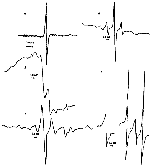
Fig.1. The ESR spectra for different rubber: a) The untreated divinyl nitrate SKN-26 and SKN-40M rubbers at room temperature ( T_{room} ); b) Brominated rubber at T_{room} ; c) Chloroprene rubber at T_{room} ; d) Chloroprene rubber at liquid nitrogen temperature; e) Isoprene rubber after being treated in the rolling machine.
