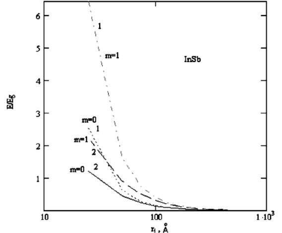
Fig.1. The dependence of the lowest quantum size levels in InSb quantum wire as function of the quantum wire radius. (1) for parabolic dispersion law. (2) for Kane's dispersion law.
