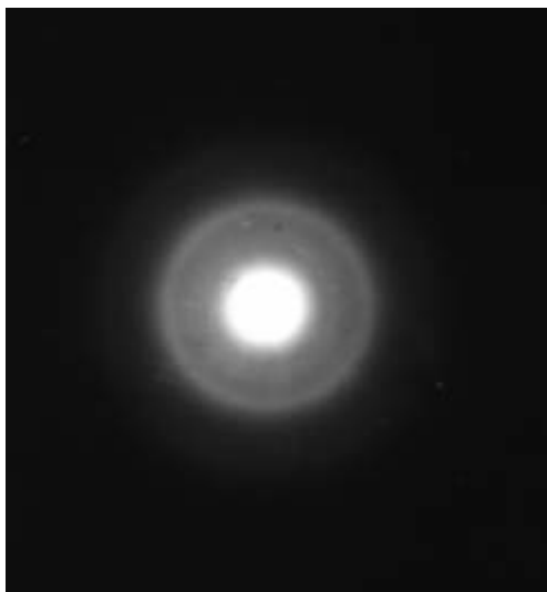
Fig. 1. Electron diffraction photograph from amorphous TlInSe 2 films.
