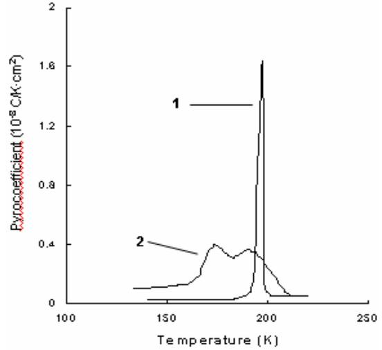
Fig. 3. The temperature dependence of the pyroelectric coefficient. Curve 1 - TlInS<sub>2</sub> crystal; Curve 2 - TlInS<sub>2</sub><Mn> crystal.
