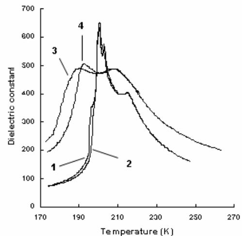
Fig.1. The dielectric constant  $\epsilon(T)$  temperature dependencies. Curves 1, 2 - the dependencies  $\epsilon(T)$  of TlInS<sub>2</sub> crystal (1-cooling; 2-heating); Curves 3, 4 - the dependencies  $\epsilon(T)$  of TlInS<sub>2</sub><Mn> crystal (3-cooling; 4-heating).
