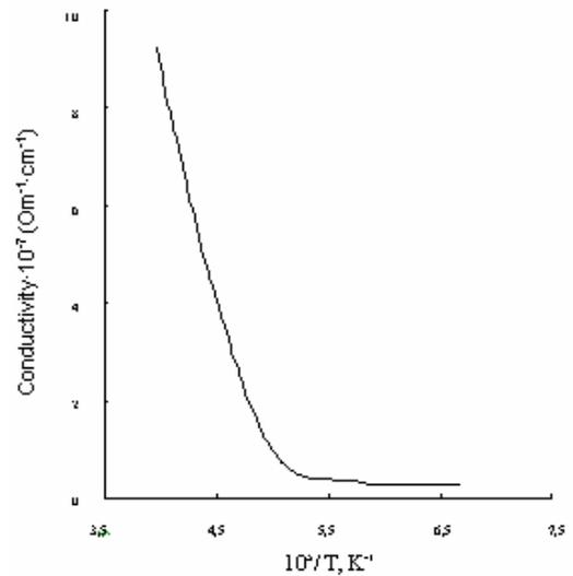
Fig. 4. The dependence of conductivity  $\sigma$  from  $1/T$  for TlInS<sub>2</sub><Mn> crystal.
