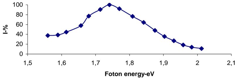
Fig. 2a. Radiation spectra of GaSe nanoparticles.
