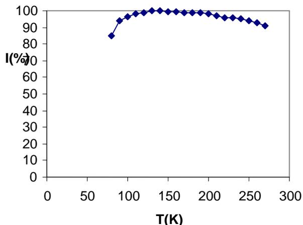
Fig.3. Temperature dependence of photoluminescence of GaSe nanoparticles.
