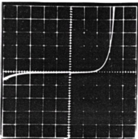
Fig.1. VAC of InP - CdS heterojunctions at T=300°K, on the point J=2mA; U=0.5V.
