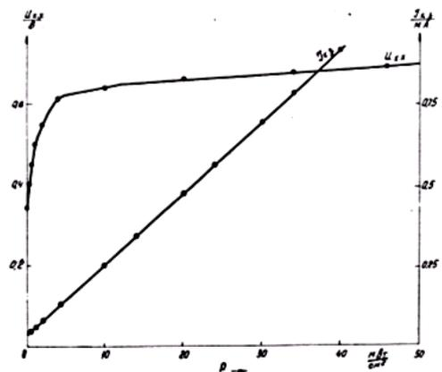
Fig.3. The dependence of open-circuit voltage  $U_{xx}$  and short-circuit photocurrent  $I_{sc}$  on the lightening.
