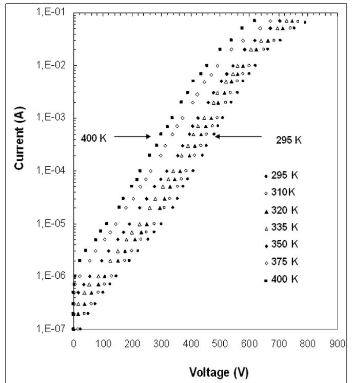
Fig. 1. Forward I-V-T characteristics of the Al/SiO<sub>2</sub>/p-Si Schottky diode.
