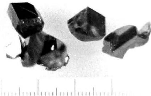
Fig. 2. The monocrystals of low-temperature modification  $\alpha\text{-Ag}_2\text{Se}$  with facets of high-temperature OCC modification.
