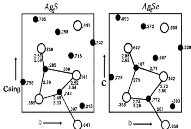
Fig.1. The structure projection of monoclinic  $\alpha$ - $\text{Ag}_2\text{S}$  and orthorhombic  $\alpha$ - $\text{Ag}_2\text{Se}$  on the [011] direction.
