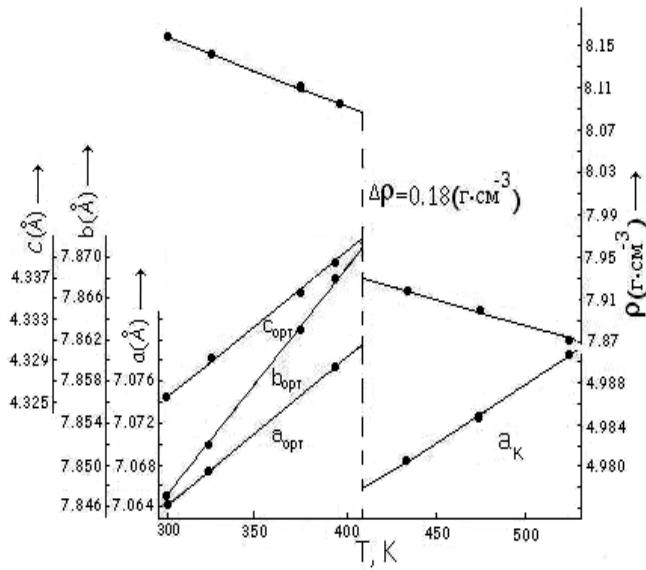
Fig.3. The temperature dependence of lattice parameters and of  $\alpha$ - and  $\beta$ -modifications density of  $\text{Ag}_2\text{Se}$ .
