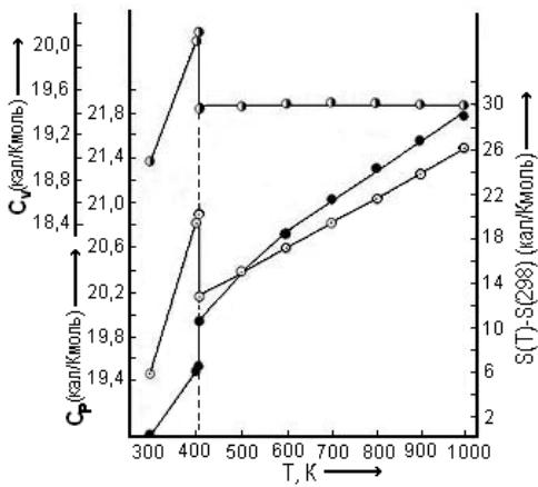
Fig.4. The temperature dependence of heat capacity of  $C_p$  and  $C_v$  entropies in temperature interval, capturing the polymorphic transformation  $\alpha \rightleftharpoons \beta$  in  $\text{Ag}_2\text{Se}$ .  $\odot$  is  $C_p$ ,  $\bullet$  is  $C_v$  and entropy.
