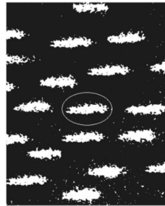
Fig.3. The longitudinal section of PbTe - NiSb eutectic surface.
