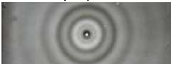
Fig.1. The electron diffraction pattern from amorphous films Yb 3(1-x)Sm x As 4 Se 9 .
