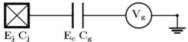
Figure 1. The simplest circuit model of a Josephson junction (JJ) including a gate voltage  $V_g$  and gate capacitance  $C_g$ . Corresponding gate charge is  $Q_g = 2en_g = C_g V_g$ .
