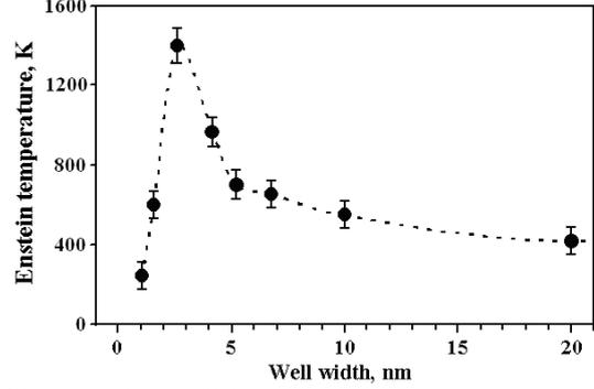
Fig.6. The dependence of Einstein's characteristic temperature  $\Theta_E$  of MQW  $Mg_{0.27}Zn_{0.73}O/ZnO$  on quantum well width  $L_w$ .
