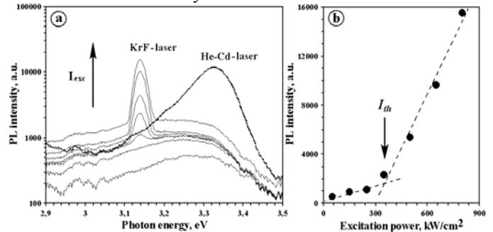
Fig.7. The PL spectra of a line 3.14 eV of MQW  $Mg_{0.27}Zn_{0.73}O/ZnO$  with a well width  $L_w = 5.2$  nm: (a) excitation by the He-Cd laser and the excimer KrF laser with pump power variation from 50 to 850  $kW/cm^2$ ; (b) dependence of PL amplitude of a line 3.14 eV of MQW  $Mg_{0.27}Zn_{0.73}O/ZnO$  on excimer KrF laser pump power.
