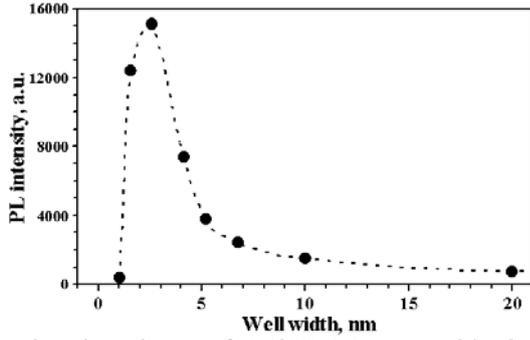
Fig.4. The dependence of MQW  $Mg_{0.27}Zn_{0.73}O/ZnO$  photoluminescence intensity on quantum well width  $L_w$ .
