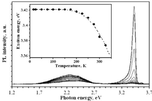
Fig.5. The PL dynamics of MQW  $Mg_{0.27}Zn_{0.73}O/ZnO$  (6 nm/2.6 nm) on temperature in the range 8-325 K. An insert illustrates the temperature dependence of exciton energy in MQW.
