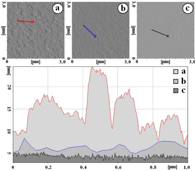
Fig.1. The surface morphology of buffer layer  $\text{Mg}_{0.27}\text{Zn}_{0.73}\text{O}$  on a sapphire substrate (00.1): (a) – before annealing, (b) – annealed at  $800^\circ\text{C}$ , (c) - annealed at  $1000^\circ\text{C}$ , and cross-section profiles of corresponding surfaces (below).
