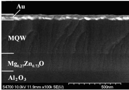
Fig.8. A SEM-image of cross-section of 20 quantum wells  $Mg_{0.27}Zn_{0.73}O/ZnO$  grown on a sapphire substrate (00.1) with a buffer layer  $Mg_{0.27}Zn_{0.73}O$ . For contrast the structure was covered by a gold film.
