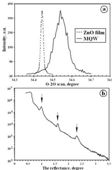
Fig.9.  $\Theta$ - $2\Theta$  scans of a ZnO film and MQW  $Mg_{0.27}Zn_{0.73}O/ZnO$  with the well width  $L_w=2.6$  nm (a). A curve of mirror reflection of MQW  $Mg_{0.27}Zn_{0.73}O/ZnO$  with the well width  $L_w=5.2$  nm.
