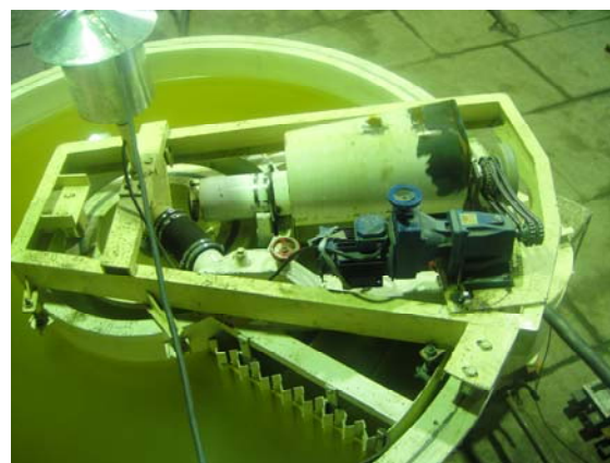
Fig.5. Circular flotation tank of pilot system
