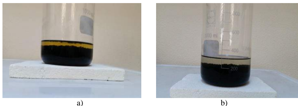
Fig. 2. The stage of purification of MWCNTs from tarry substances by extraction method: a) MWCNTs suspension with solvent during extraction; b) MWCNTs suspension with solvent after extraction.
