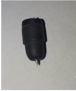
Fig. 3. A needle made of nickel-chromium wire, impregnated with InSb, is placed inside a graphite container.
