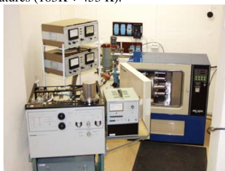
Figure 11. "Edelweiss-001" standardized unit for testing hydrogen sensors
