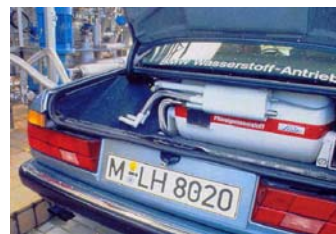
Figure 1. A cryogenic hydrogen tank in the hydrogen car trunk (D. Orlov. Heat will save the world // Around the world, 2003, p. 67–73)
