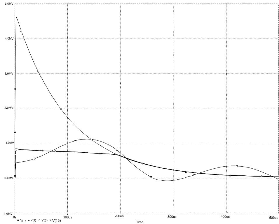
Fig. 2: Surge voltage on the arresters and on the HV neutral of the transformer
