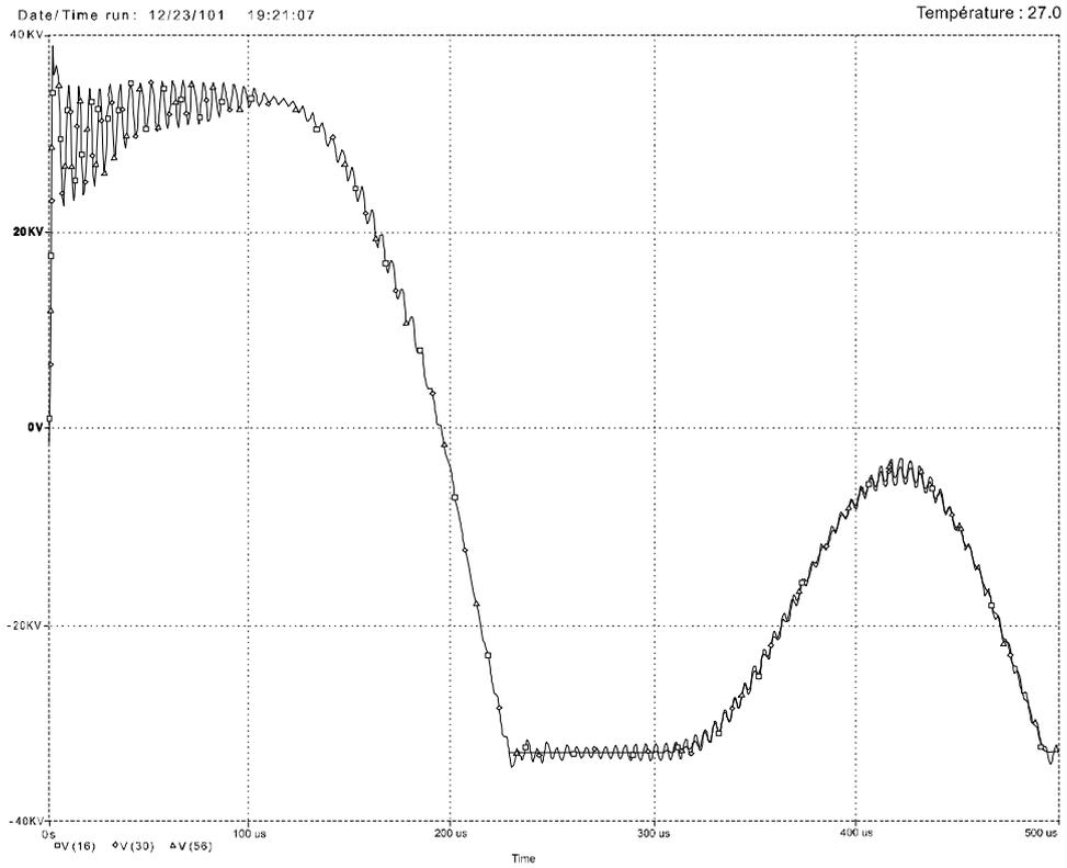
Fig.4c : The primary neutral is earthed with emplacement of the arrester at the N-side
