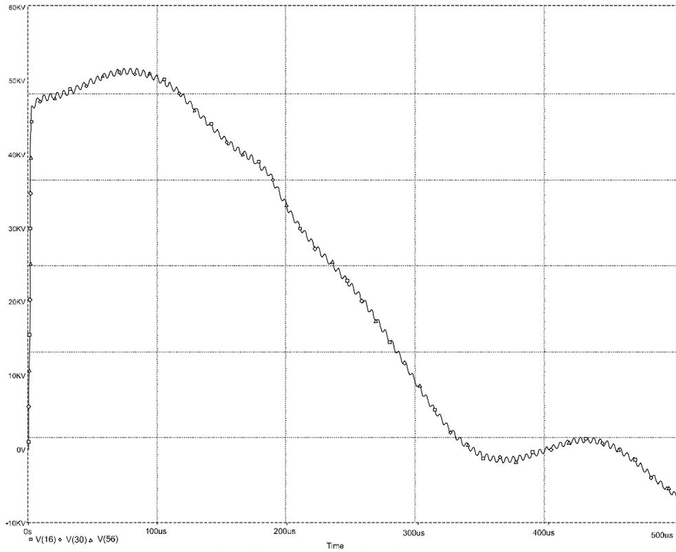
Fig. 4b : The primary neutral is earthed without arresters
