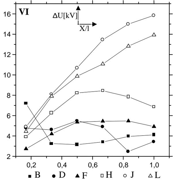
Figure 5 :Potential gradients of the relative distance . **I, III,** et **V** with arresters at the low voltage side **II,IV** and **VI** with arresters at the low voltage.
