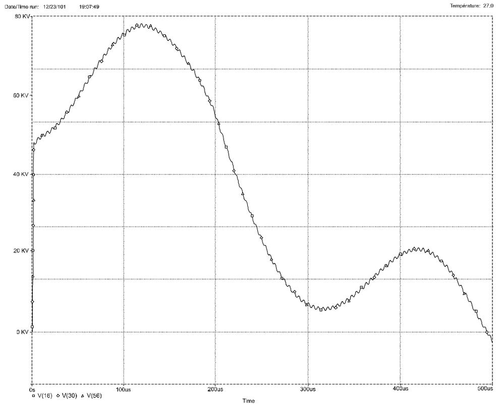
Fig.4 : Surevoltage on the LV winding connected in  $\Delta$  type
