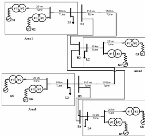
Figure 5. Multi-machine system for test and simulation
