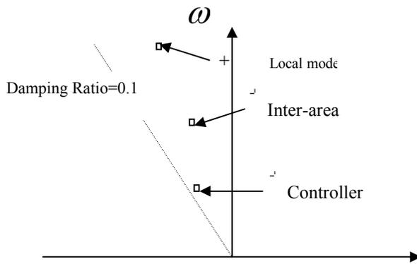
Figure 3. Objective of the optimization-based tuning: +: eigenvalues before the optimization, ·: eigenvalues after the optimization
