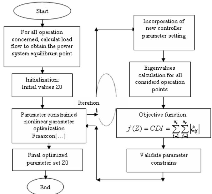
Figure 4. Flowchart of optimization-based coordinated tuning
