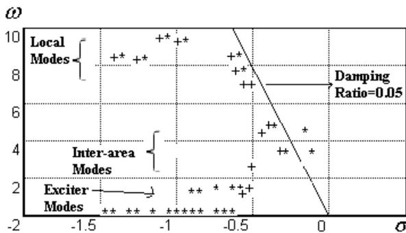
Figure 8. Location change of eigenvalues : \* eigenvalues before optimization , + eigenvalues after optimization
