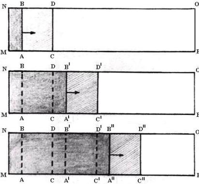
established in the first microscope, where  $\Delta T_2<\Delta T_3$ , and the measurement was repeated for the region  $A''B''C''D''$ , etc. Between measurement regions of the investigated crystal there were regions  $MNAB, CDA'B', C'D'A'B'$ , etc. since the phase separation boundary moved a certain distance during the time to transfer the crystal from one microscope to the other and establish the fixed temperature. This is illustrated in Fig.2.
