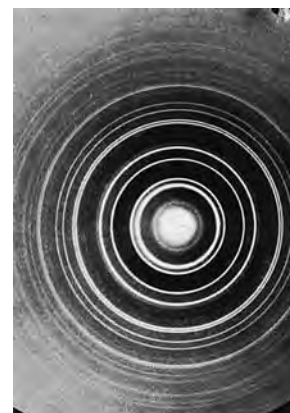
Figure 5.7 Diffraction of 50-kV electrons from a film of \text{Cu}_3\text{Au} . The alloy film was 400 \text{ \AA} thick. (Courtesy of the late Dr. L. H. Germer)
