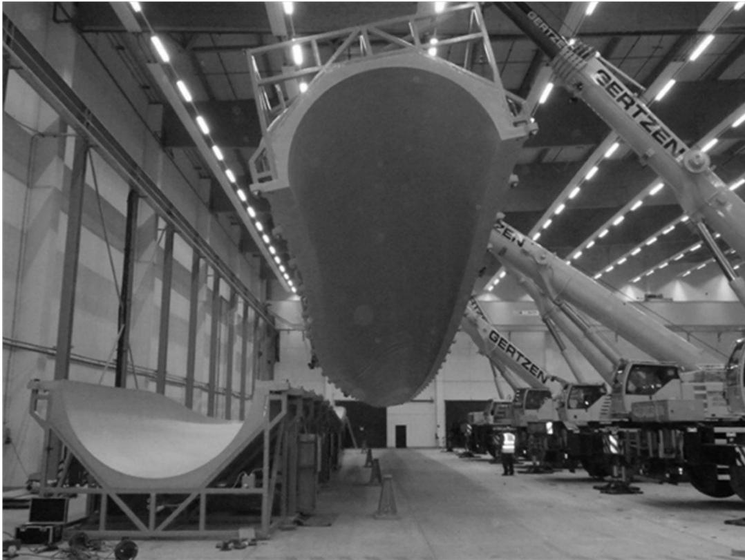
Figure 17: Mould for a 52m wind turbine blade (source: Bright Composites)
