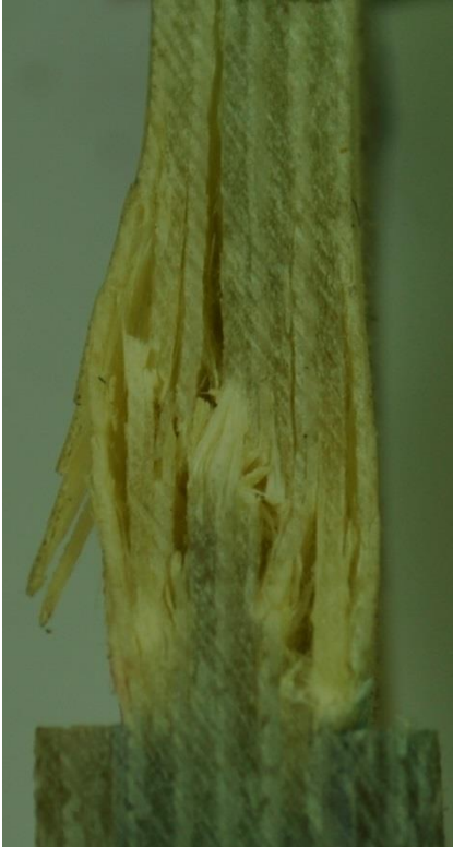
Figure 28: Buckling of plies and secondary delamination
