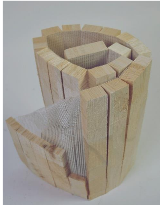
Figure 16: Core material with grooves (source: WMC)
