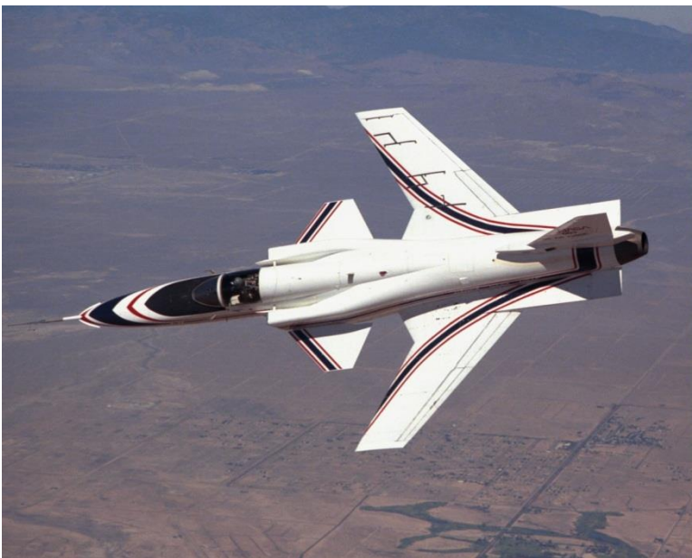
Figure 36: Aircraft in which a coupling effect has been deliberately 'built-in'
