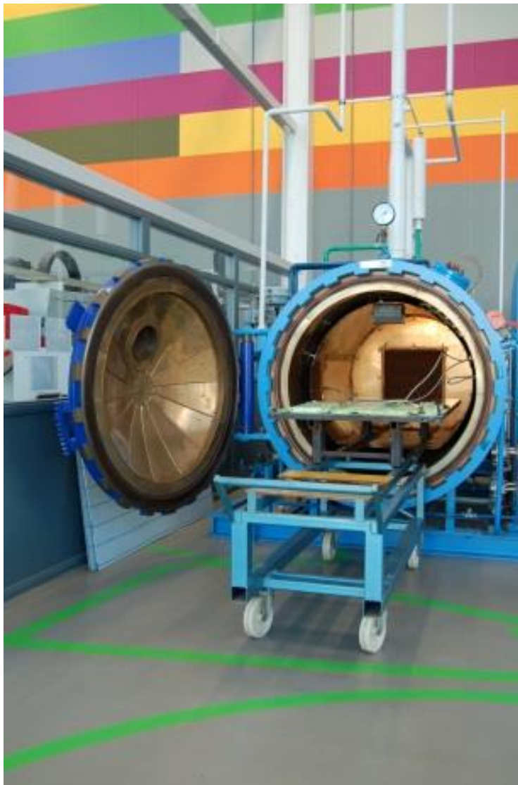
Figure 25: Autoclave at the composites lab, INHolland, Delft
