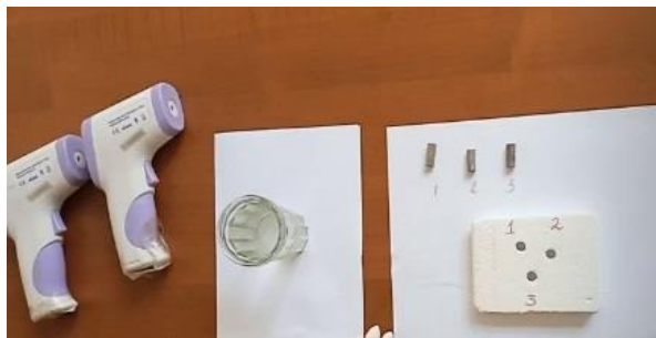
Fig. 2. Heat sink: 1- pictometer, 2- samples, 3- water cup, 4- penoplast holder with low thermal conductivity.
