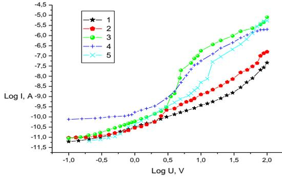
Fig. 1. The volt-ampere characteristics of  $Se_{95}Te_5$  composition with samarium impurity: 1 is  $Se_{95}Te_5$ ; 2 is  $Se_{95}Te_5Sm_{0.05}$ ; 3 is  $Se_{95}Te_5Sm_{0.1}$ ; 4 is  $Se_{95}Te_5Sm_{0.5}$ ; 5 is  $Se_{95}Te_5Sm_1$  taken at room temperature on films of thickness  $3\mu m$ .
