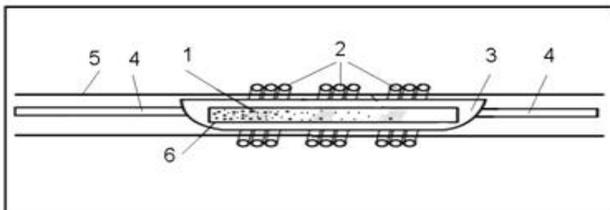
Fig.1. The scheme of installation of cascade zone melting. 1 is crucible with substance; 2 are heaters; 3 is vacuum-degassed ampoule; 4 are holders; 5 is guide tube.
