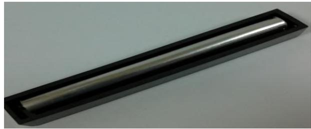
Fig.2. The boat from carbon-base glass for aluminum zone melting.
