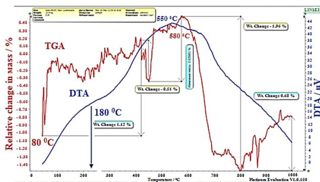
Fig. 4 Derivatogram of mass loss (TGA) and heat fluxes (DTA) curves taken from the sample Gobu / MWCNTs.
