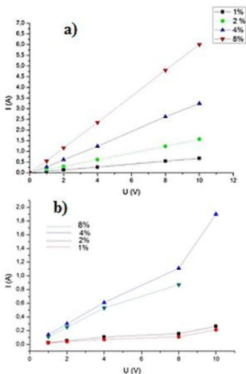
Fig. 2 Current - voltage characteristics of nanocarbon-ceramic composites based on: a) AT/MWCNTs; b) Gobu / MWCNTs.
