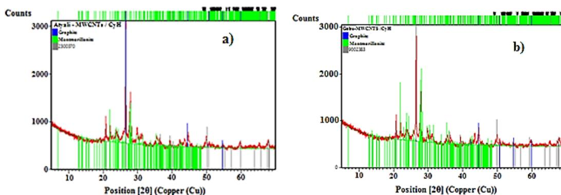
Fig. 5 X-ray diffractograms of the samples: a) AT / MWCNTs; b) Gobu / MWCNTs.
