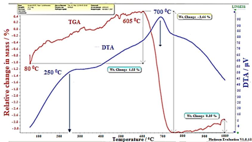
Fig. 3 Derivatogram of mass loss (TGA) and heat fluxes (DTA) curves taken from the sample AT / MWCNTs
