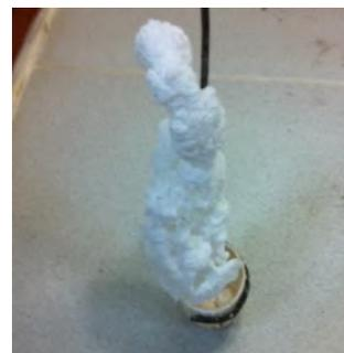
Fig. 1. SrAl<sub>2</sub>O<sub>4</sub>:Eu<sup>2+</sup> nanosized powder synthesized by combustion method.
