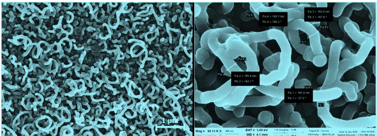
Fig. 3 SEM picture of the CNTs deposited on Fe covered c-plane sapphire substrate (left). On the right the magnification is enlarged. (SEM investigations were done at Institute of Materials for Electronics and Magnetism, in Italy)
