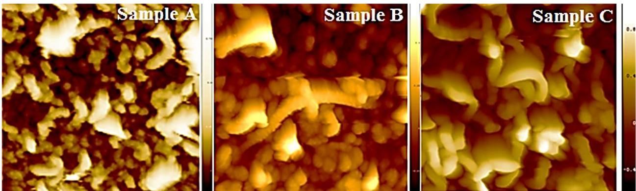
Fig. 2a-c show the atomic force microscopy topography forward 2D images of CNTs.
