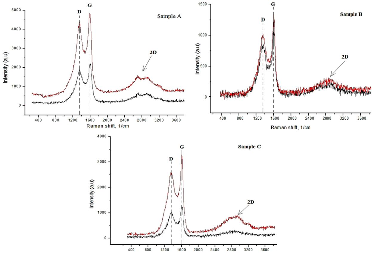
Fig. 1. Raman spectrum from a MWCNTs samples grown on sapphire substrate (black- at 4mW red- at 8 mW laser excitation powers).
