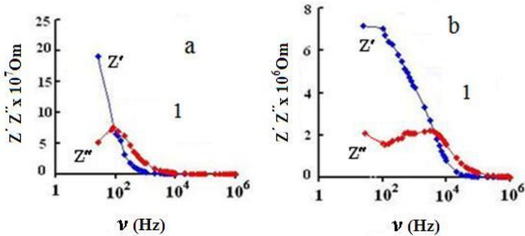
Fig.1. The frequency dependences of real ( $Z'$ ) and imaginary ( $Z''$ ) of impedance component for TlGaSe<sub>2</sub> sample. *a* figure are the measurements carried out before  $\gamma$ - irradiation and *b* figure are the measurements after  $\gamma$ - irradiation.
