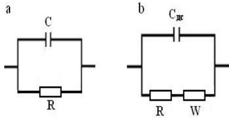
Fig.3. Equivalent circuit (**a** is before  $\gamma$  – irradiation, **b** is after it) for electrode with capacity of  $C_{DL}$  double layer,  $W$  is Warburg diffuse impedance,  $R$  is sample resistance.
