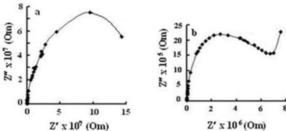
Fig.2. The diagram on complex plane ( $Z''-Z'$ ) obtained on the base of fig.1. The figure *a* are the measurements carried out before  $\gamma$ - irradiation, figure *b* are the measurements after  $\gamma$ -irradiation.
