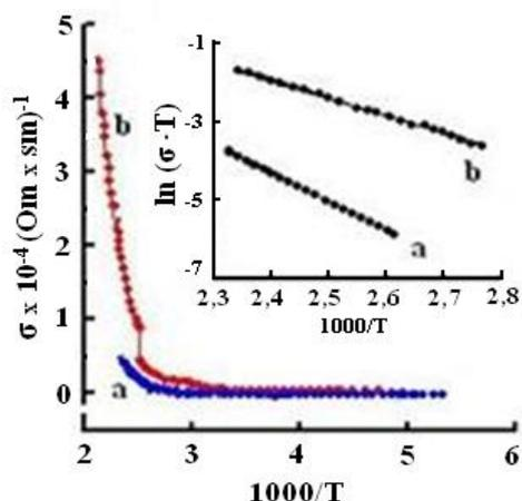
Fig.4. Temperature dependence of TlGaSe<sub>2</sub> crystal conduction in Arrhenius coordinates.  $\ln(\sigma \cdot T)$  dependence on  $1000/T$  is given in insert. **a** curve represents the measurement results carried out before gamma irradiation, **b** curve represents the measurements after it.
