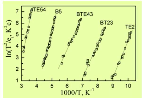
Fig. 2. - Rate of charge carrier emission from deep level traps in TIInS<sub>2</sub>:La as function of temperature by taking into account  $T^2$  correction. Solid lines represent the fitting to experimental data.
