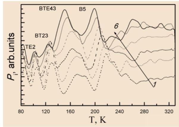
Fig. 1. - PICTS spectra of TIInS<sub>2</sub>:La corresponding to the thermal emission rate: 1) 2200 s<sup>-1</sup>; 2) 1350 s<sup>-1</sup>; 3) 770 s<sup>-1</sup>; 4) 408 s<sup>-1</sup>; 5) 213 s<sup>-1</sup>; 6) 108 s<sup>-1</sup>; 7) 54 s<sup>-1</sup>. The spectra are normalized to the height of the maximal peak and shifted along Y -axis/
