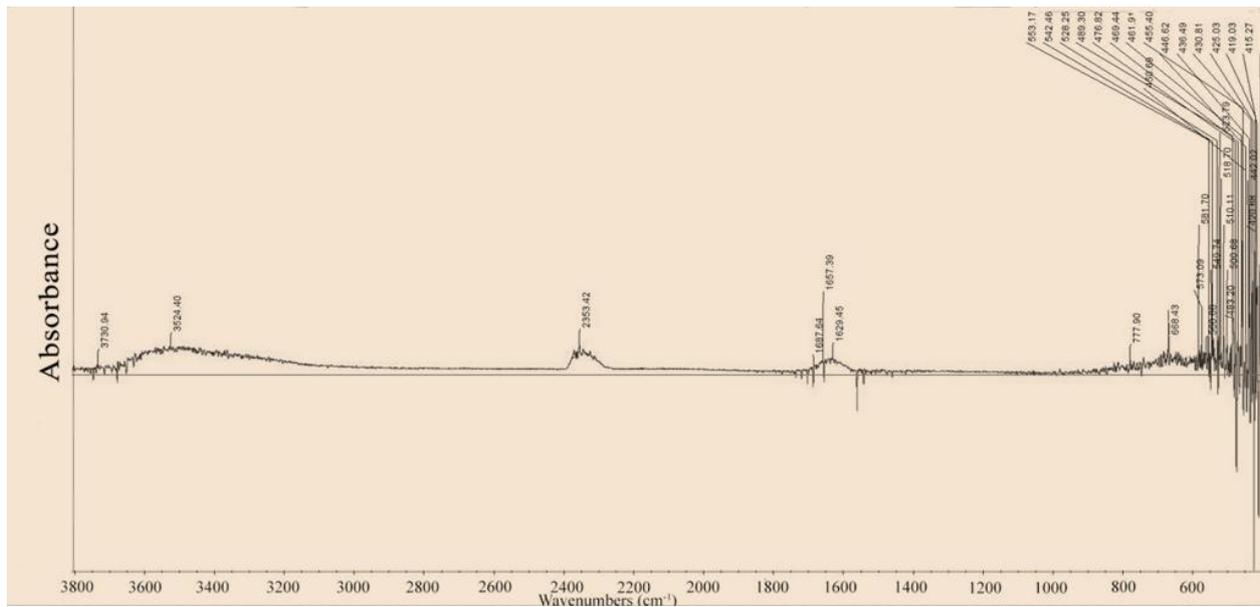
Fig.5. FTIR spectrum of gaseous products of the oxidation-thermal destruction process of f- MWCNTs at 370 °C.
