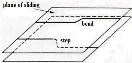
Fig. 2. Steps and bends on dislocations [8]. The cases when dislocation is in two neighbor plains of sliding, bends (blades) and another type which is step, are possible.
