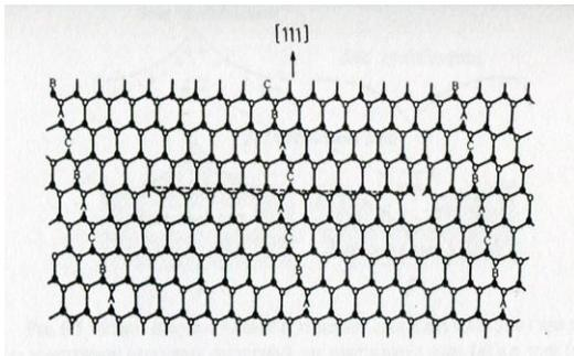
Fig.3. The cell is the type in direction of dislocation wire on atomic structure of 60% split dislocation in lattices by diamond type: the atoms of the similar elements in single crystals of IV group are marked by black and white circles. The detail explanation is in [8].
