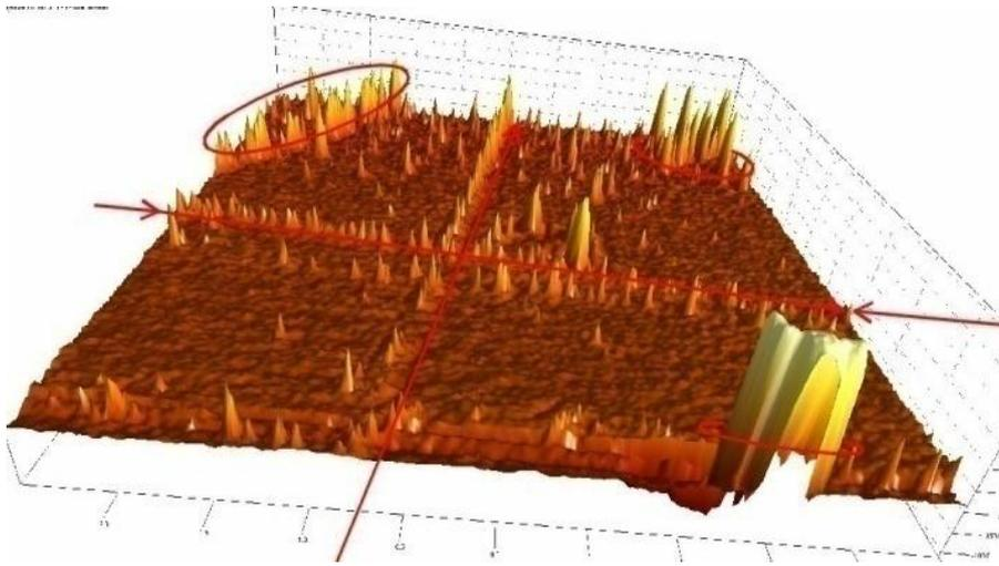
Fig.5. The dislocation structure obtained by us in  $Bi_2Te_3$  on (0001) surface (the nano-objects in the form of localized nano-islands are given on top left and right in upper part of the figure) (macroscope is AFM - BRUKERNANO)
