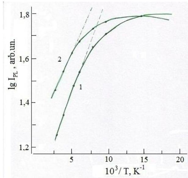
Fig. 2. Temperature quenching of photoluminescence intensity of ZnGa<sub>2</sub>S<sub>4</sub> for emission bands 1- 440 nm, 2- 540 nm
