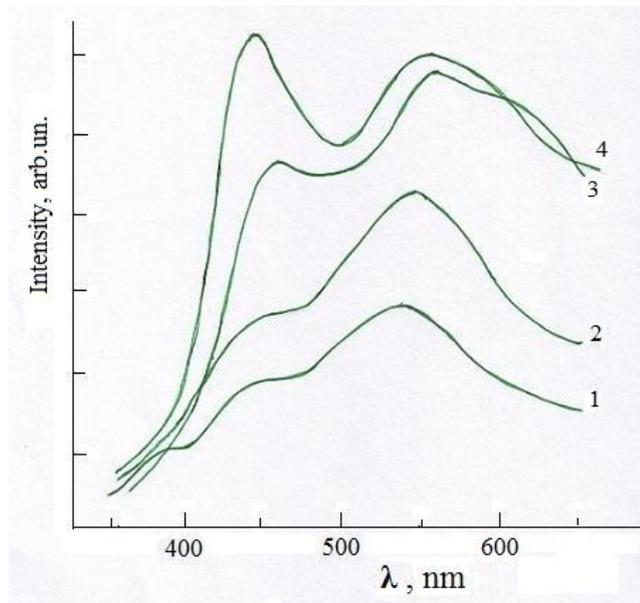
Fig. 1 Photoluminescence spectra of ZnGa<sub>2</sub>S<sub>4</sub> at 1- 300, 2- 202, 3- 110, 4- 74 K
