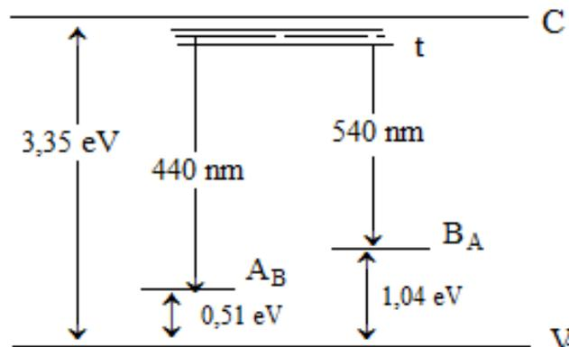
Fig. 3. Scheme of local states and electron transitions in ZnGa<sub>2</sub>S<sub>4</sub>
