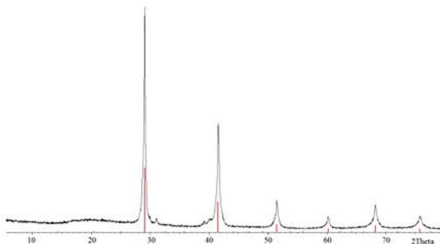
Fig. 1. The X-ray diffractogram of  $(\text{AgSbTe}_2)_{0.8}(\text{PbTe})_{0.2}$
