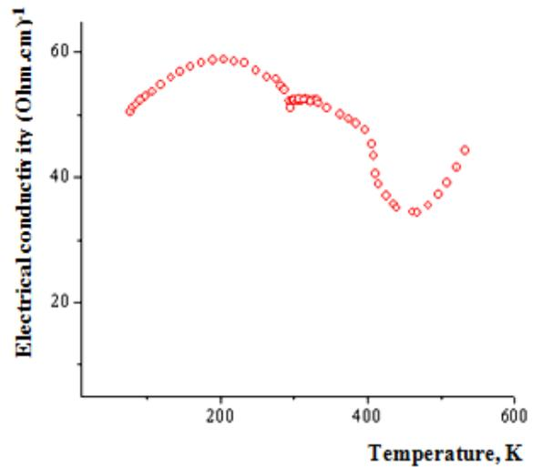
Fig. 2. The temperature dependences of the resistivity of  $(\text{AgSbTe}_2)_{0.8}(\text{PbTe})_{0.2}$
