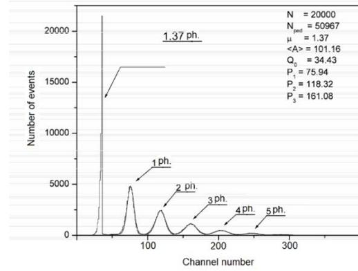
Fig. 3. MAPD spectrum (at fixed T and  $U_{bias}$ ). Designations:  $N$ ,  $N_{ped}$  - respectively the total number of events and the number of events in the pedestal;  $\mu$  is the average number of photoelectrons;  $\langle A \rangle$  - average value of the histogram;  $Q_0$  is the position of the pedestal,  $P_1$ ,  $P_2$ ,  $P_3$  are the positions of the peaks of the 1st, 2nd and 3rd photoelectrons, respectively.
