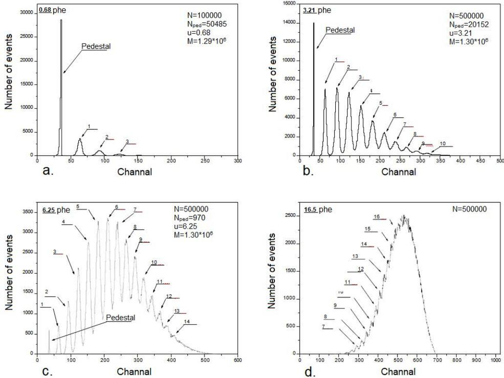
Fig. 4. Spectra obtained with MAPD ( $T = 220C$ ,  $U_{bias} = 60V$ ). Designations:  $N$  - total number of events, bold and underlined numbers,  $\mu$  - average number of photoelectrons,  $M$  - gain determined from the peak of the first photoelectron.
