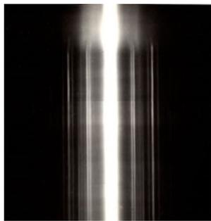
Fig. 1. Kinematic electron diffraction pattern showing  $\text{TlIn}_{0.93}\text{Sn}_{0.07}\text{Se}_2$  crystallization at temperature 450K.
