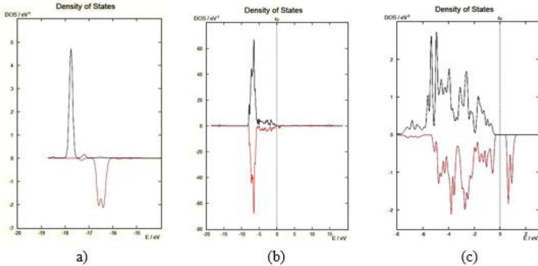
Fig. 4. Partial densities of states of a) s state-18<sup>th</sup> oxygen atom near of vacancy, b) d-state- Cu atom, c) density of states of CuZn<sub>17</sub>O<sub>18</sub>
