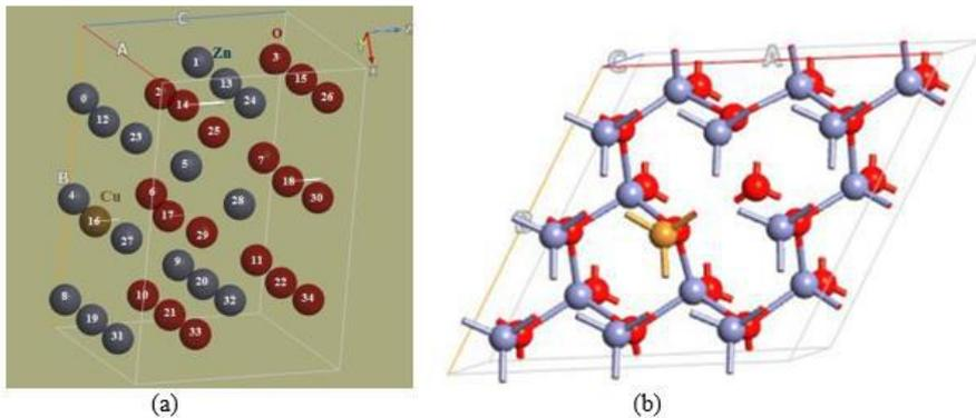
Fig. 3. The atom structure  $\text{Zn}_{16}\text{O}_{18}\text{Cu}$  with Zn (a),(b) vacancy.
