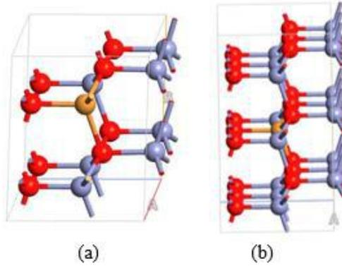
Fig. 2. The models of: (a)  $\text{Cu}_{0.125}\text{Zn}_{0.875}\text{O}$  supercell, (b)  $\text{Cu}_{0.056}\text{Zn}_{0.944}\text{O}$  supercell.
