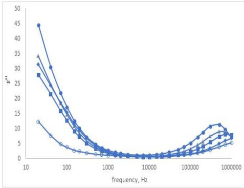
Fig. 3. The frequency dependence of imaginary part of barium titanate–oleic acid mixture: empty circles–100nm BaTiO<sub>3</sub>; filled circles–200nm BaTiO<sub>3</sub>; triangles–300nm BaTiO<sub>3</sub>; squares–400nm BaTiO<sub>3</sub>; rhombs–100n m BaTiO<sub>3</sub>.
