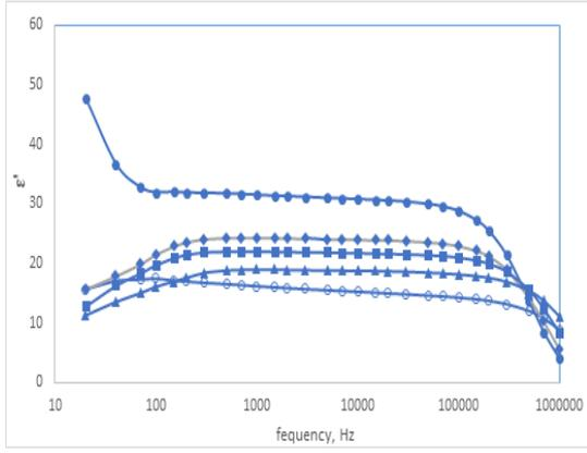
Fig. 2. The frequency dependence of real part of barium titanate – oleic acid mixture: empty circles–100nm BaTiO<sub>3</sub>; filled circles–200nm BaTiO<sub>3</sub>; triangles–300nm BaTiO<sub>3</sub>; squares– 400nm BaTiO<sub>3</sub>; rhombs–100nm BaTiO<sub>3</sub>.
