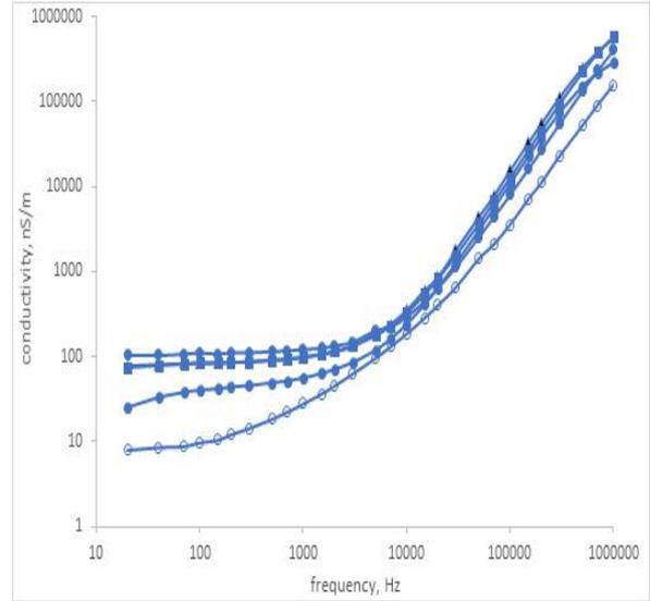
Fig. 4. The frequency dependence of electric conductivity of barium titanate–oleic acid mixture: empty circles–100nm BaTiO<sub>3</sub>; filled circles–200nm BaTiO<sub>3</sub>; triangles–300nm BaTiO<sub>3</sub>; squares–400nm BaTiO<sub>3</sub>; rhombs–100nm BaTiO<sub>3</sub>.
