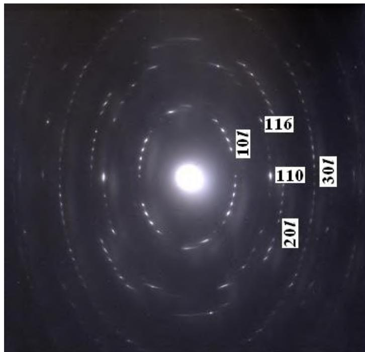
Fig.1. The rotation electron-diffraction pattern of  $\text{Fe}_{0.75}\text{Ga}_{0.25}\text{InS}_3$  ( $\varphi=40^\circ$ ,  $\omega=45^\circ$ ) single crystal of 2H- polytype. The single-crystal film is evenly placed on CH plane.
