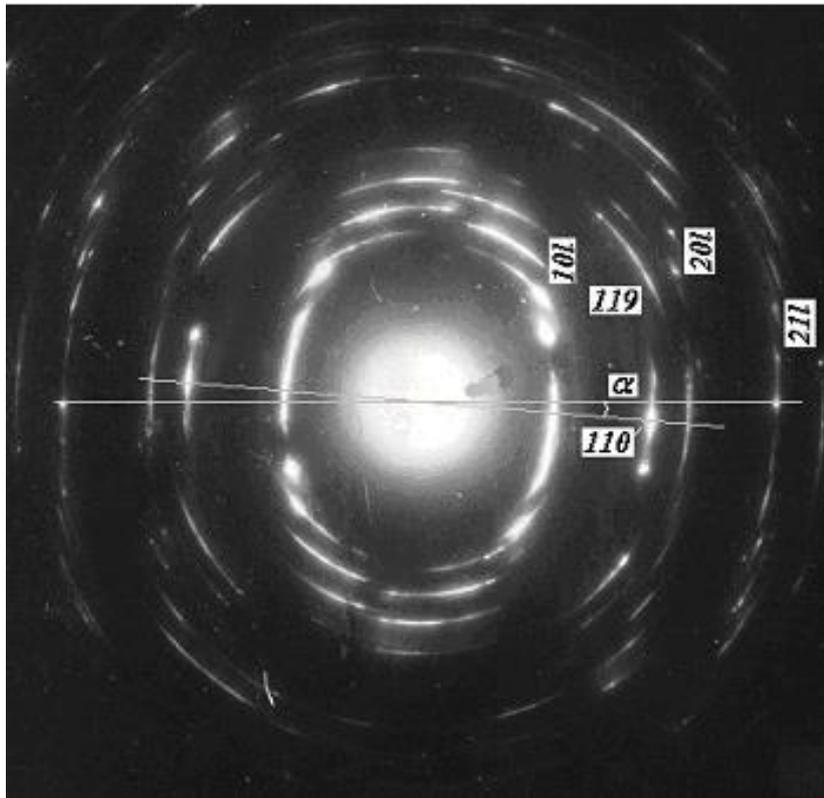
Fig.3. The rotation electron-diffraction pattern of  $\text{Fe}_{0.25}\text{Ga}_{0.5}\text{In}_{1.25}\text{S}_3$  ( $\varphi=55^\circ$ ,  $\omega=60^\circ$ ) single crystal of 3R polytype. The single-crystal film is located under  $\theta$  angle to CH plane. The reflection tilt 110 on  $\alpha$  angle from direction of CH tilt axis is connected with initial tilt of film on  $\theta$  angle.
