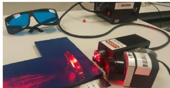
Fig. 4. A picture of temperature measurement set-up with infrared/thermal camera for the deliberately colored Zerdine phantom.
