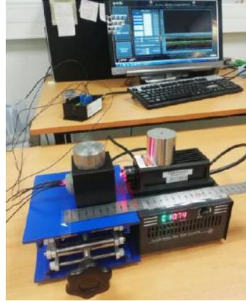
Fig. 2. Internal temperature measurement set-up.
