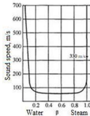
Fig.3. The curve of the dependence of velocity of sound in homogenous two-phase mixture on volume state of phases water–steam.
