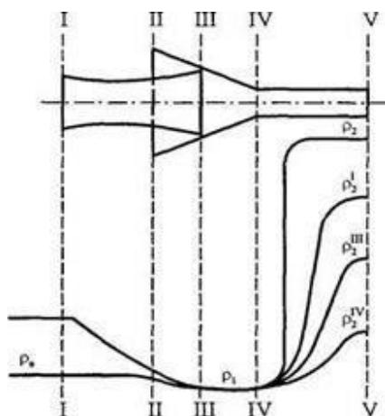
Fig.5. The graphs of pressure distribution inside apparatus.
