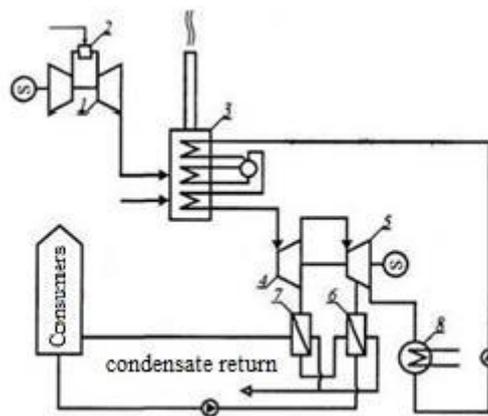
Fig.1. The scheme of steam-gas TPP: 1 is gas-turbine plant; 2 is combustion chamber; 3 is boiler-utilizer; 4 is steam turbine, part of high pressure; 5 is steam turbine, part of low pressure, 6 is means water heater of low pressure, 7 is means water heater of high pressure, 8 is condenser.
