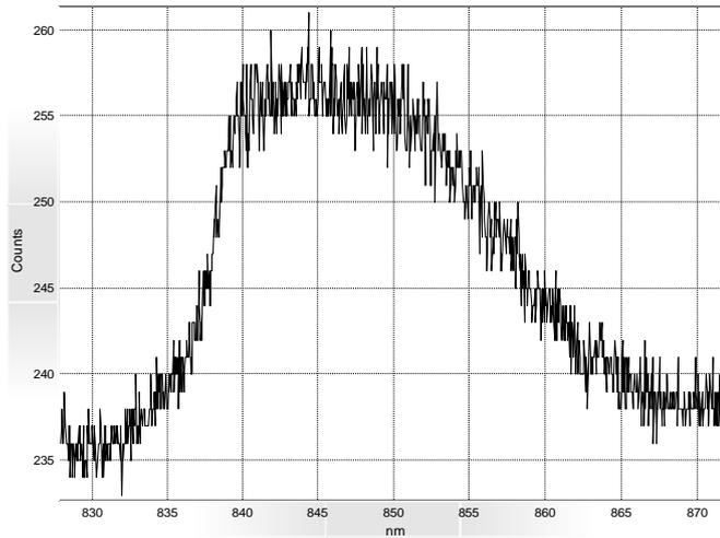
Fig. 2. Emission spectrum of low-resistance thin CdS films upon single-photon excitation by the 3rd harmonic of a Nd:YAG laser ( $\lambda = 355$  nm).
