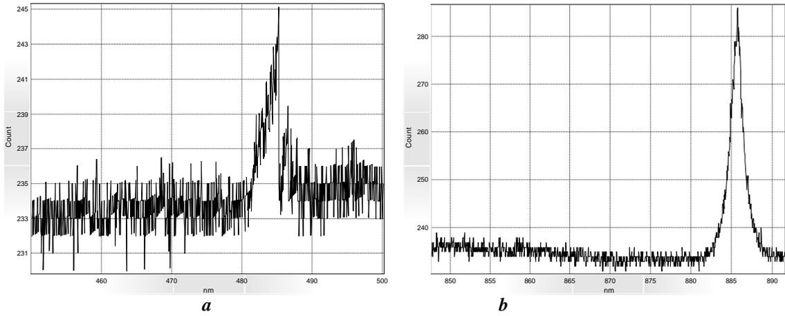
Fig. 1. Emission spectrum of thin CdS films upon single-photon excitation by the 3rd harmonic of a Nd:YAG laser ( $\lambda = 355$  nm).
