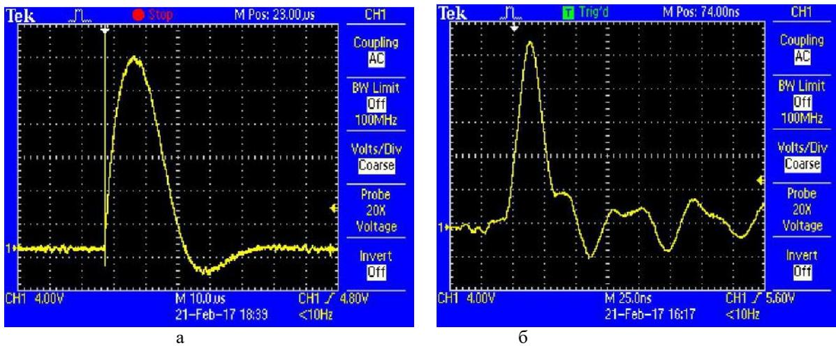
Fig. 3. Photocurrent kinetics upon excitation of thin CdS films under single-photon excitation by the 3rd harmonic of the Nd:YAG laser ( $\lambda = 355$  nm).
