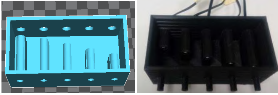
Fig. 2. Temperature Measurement Systems and NTC-Type Thermistor Temperature Sensors.
