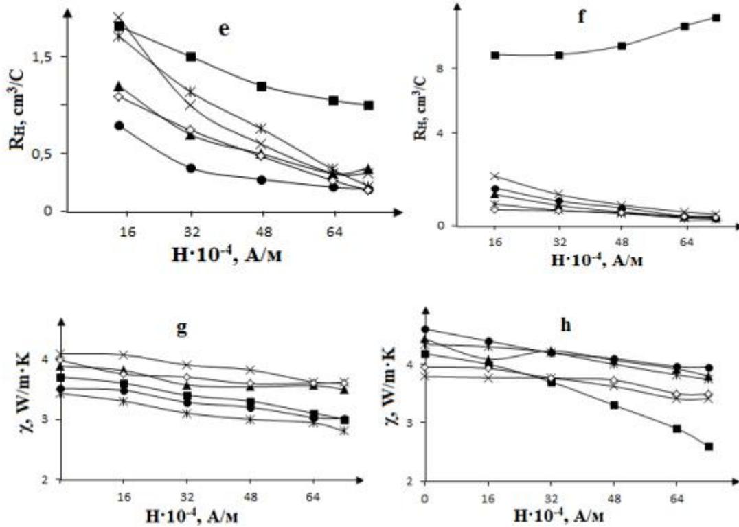
Fig. 3. Dependences of electrical conductivity ( $\sigma$ ), thermo-e.m.f. ( $\alpha$ ), Hall ( $R_H$ ) and thermal conductivity ( $\chi$ ) coefficients of the extruded samples of  $\text{Bi}_{0.85}\text{Sb}_{0.15}$  solid solution with various sizes of particles before (a, c, e, g) and after (b, d, f, h) heat treatment on magnetic fields intensity at  $\sim 77$  K. The designations are the same as in Fig.1
