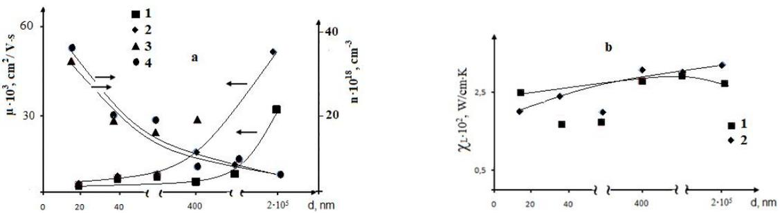
Fig. 2. Dependences of the concentration ( $n$ ), mobility ( $\mu$ ) of current carriers (a) and the phonon part of thermal conductivity ( $\chi_L$ ) (b) of nanostructured extruded samples of the  $Bi_{0.85}Sb_{0.15}$  solid solution on the particle size at  $\sim 77$  K. Fig. a, curves 1,3 - unannealed samples, 2,4 - annealed samples, Fig. b- 1- annealed samples, 2- unannealed samples.
