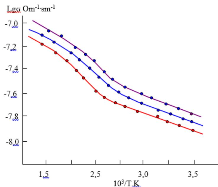
Fig. 4. The dependence of electrical conductivity of solid solution alloys (SrSe)<sub>1-x</sub>(Ga<sub>2</sub>Sr)<sub>x</sub> (x=0.01; 0.02; 0.03) on composition and temperature was studied. 1-1 mol. %, 2-2 mol. %, 3-3 mol. % Ga<sub>2</sub>Sr.
