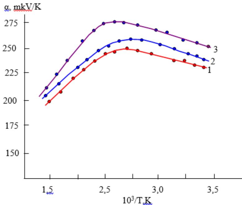
Fig. 5. Dependence of thermo-EMF of solid solution alloys  $(\text{SrSe})_{1-x}(\text{Ga}_2\text{Sr})_x$  ( $x=0.01; 0.02; 0.03$ ) on composition and temperature. 1-1 mol. %, 2-2 mol. %, 3-3 mol. %  $\text{Ga}_2\text{Sr}$ .
