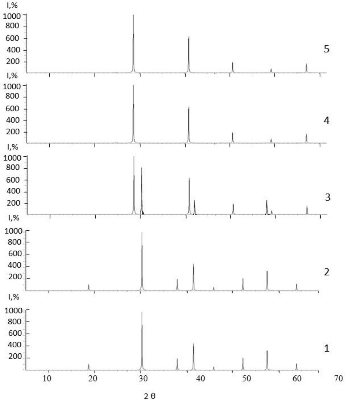
Fig. 2. X-ray diffraction patterns of alloys of the Ga<sub>2</sub>Sr-SrSe system.
