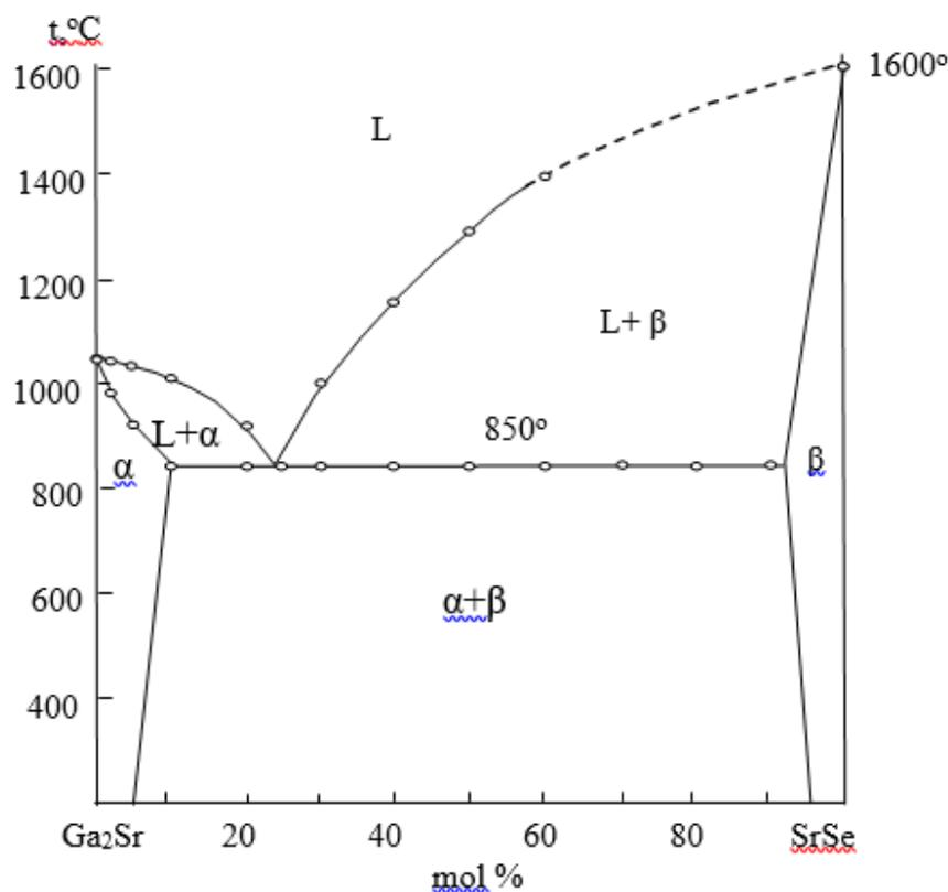
Fig. 3. T-x phase diagram of the Ga<sub>2</sub>Sr–SrSe system.
