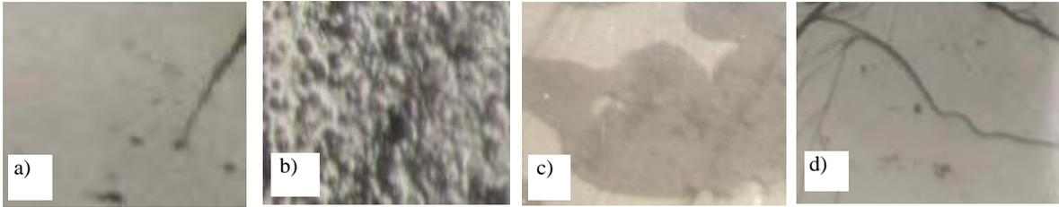
Fig. 1. Microstructures of alloys of the Ga<sub>2</sub>Sr-SrSe system. a) -5, b) -25, c) -60, d) -96.5 mol % SrSe
